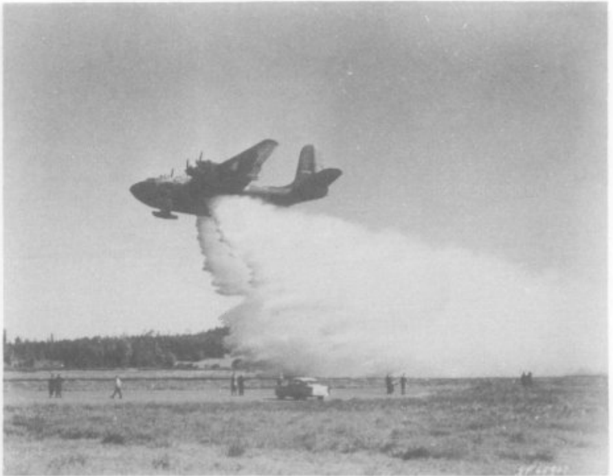
Martin JRM-1 Mars dropping approximately 8,000 gallons of water in a test of its fire-fighting ability. Martin Marietta.
